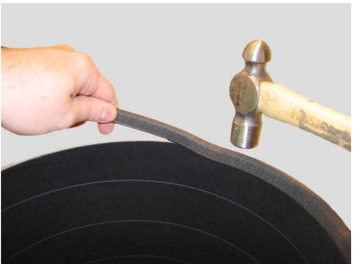
Tapping end trim onto a BlackLite tube.
