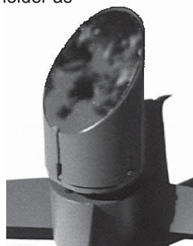
Figure 1: Shroud-mounted secondary mirror
